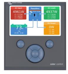
Color Control panel, showing a **PV** application
